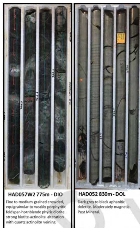
Figure 9: Photographs of the two intrusive units at Haverion (Source: Newcrest).
