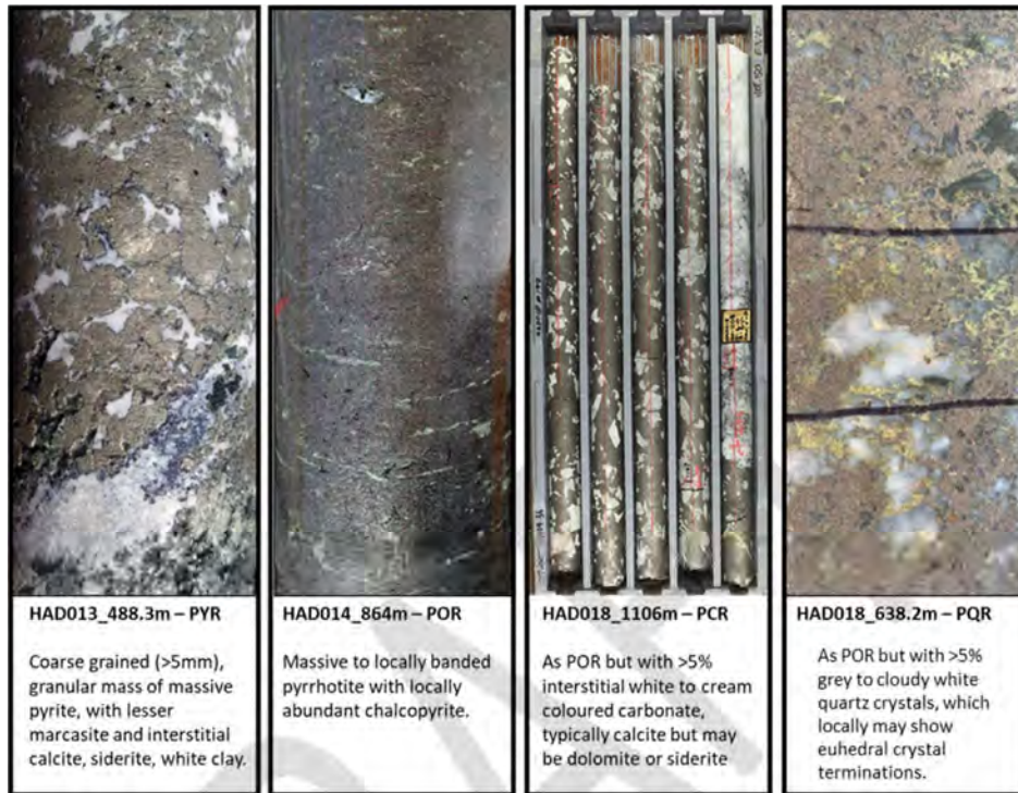
Figure 3: Photograph examples of the sulphide units at Havieron (Newcrest 2020).
